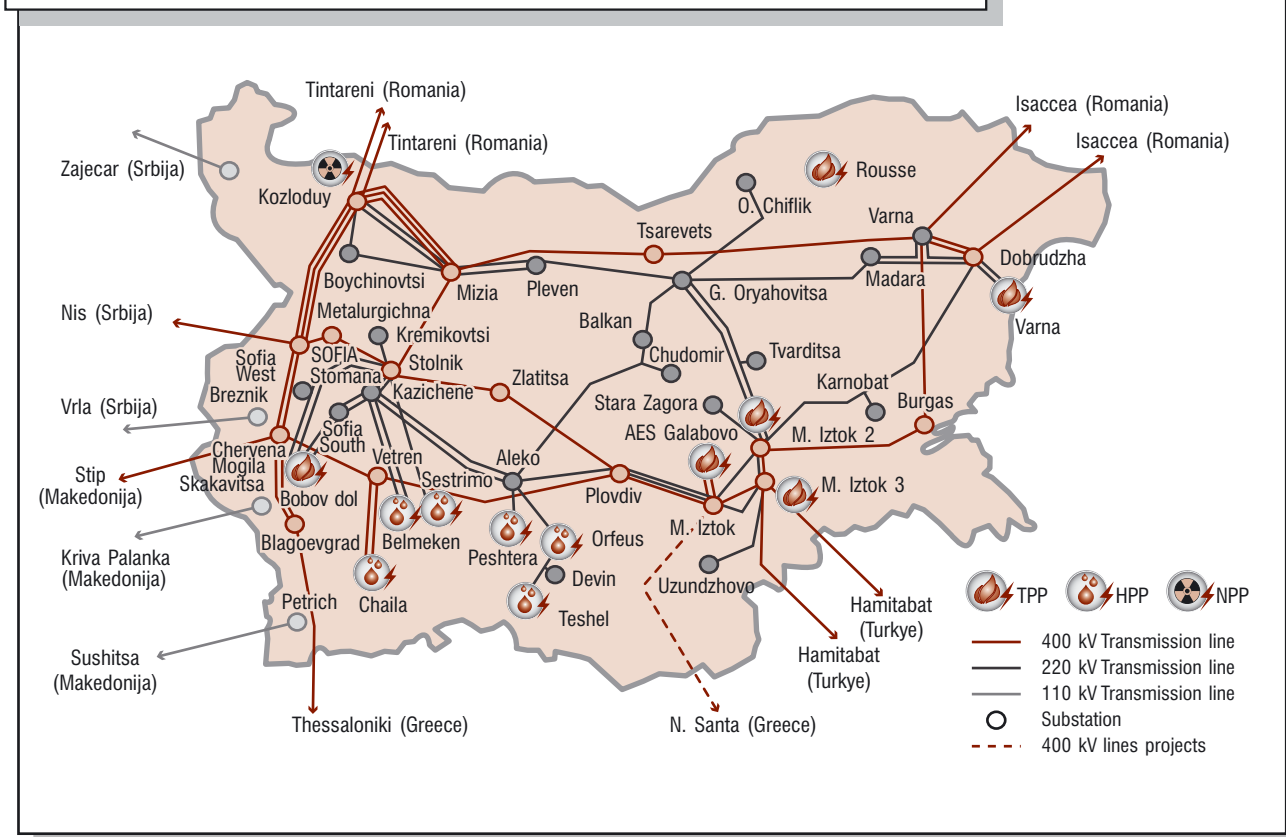
Figure 12. Map of the Electricity Grid of Bulgaria
