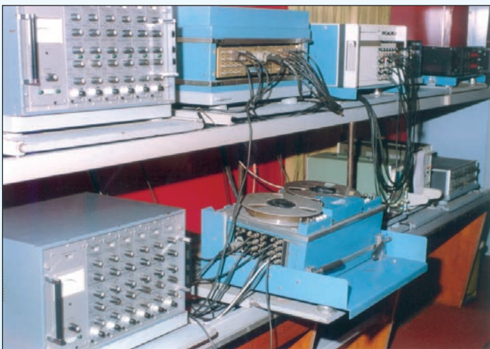
Fig. 3. Measuring equipment for testing freight wagons
