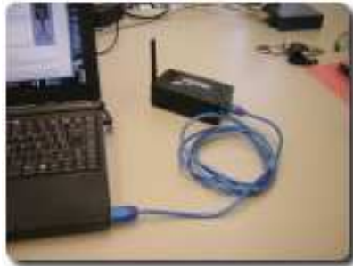
Service developed which extracts sensor data from Squidbee devices (Zigbee enabled)
