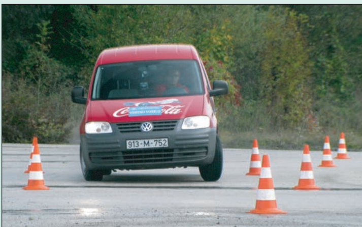
Figure 1. Stability test of the light duty vehicle during curve maneuver
